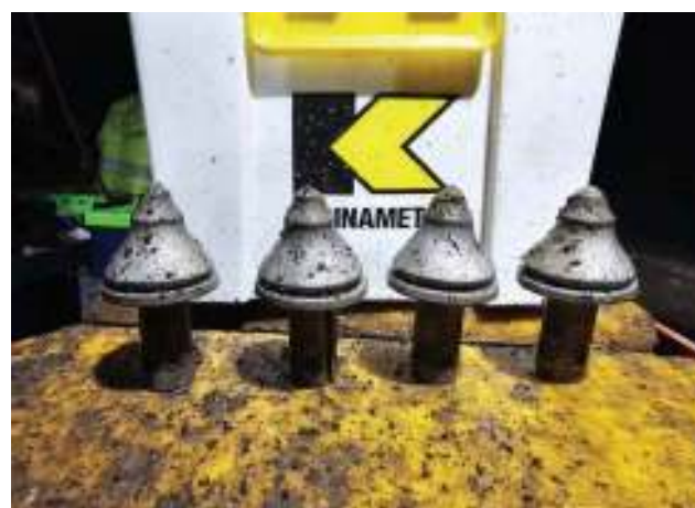
Kennametal RK52 picks at job completion. Body shape creates extra clearance under the tip and extra slope for holder protection.
